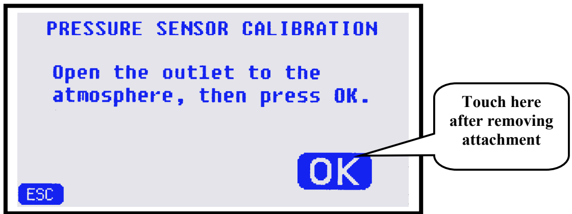
Figure 16 – Setting atmospheric value.
