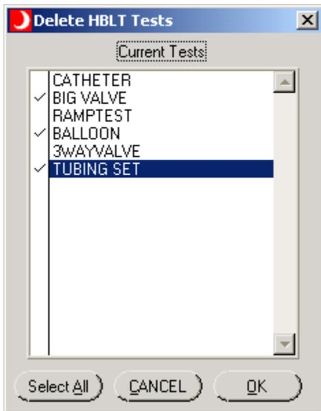
Use this panel to delete groups or all files from the HBLT. This function is helpful when downloading a new test set. The single delete mode on the Test Parameters panel uploads all the HBLT tests after each delete to insure Pressure Manager reflects the correct HBLT test status. This panel deletes all checked tests and then does a single upload of all the HBLT tests.
