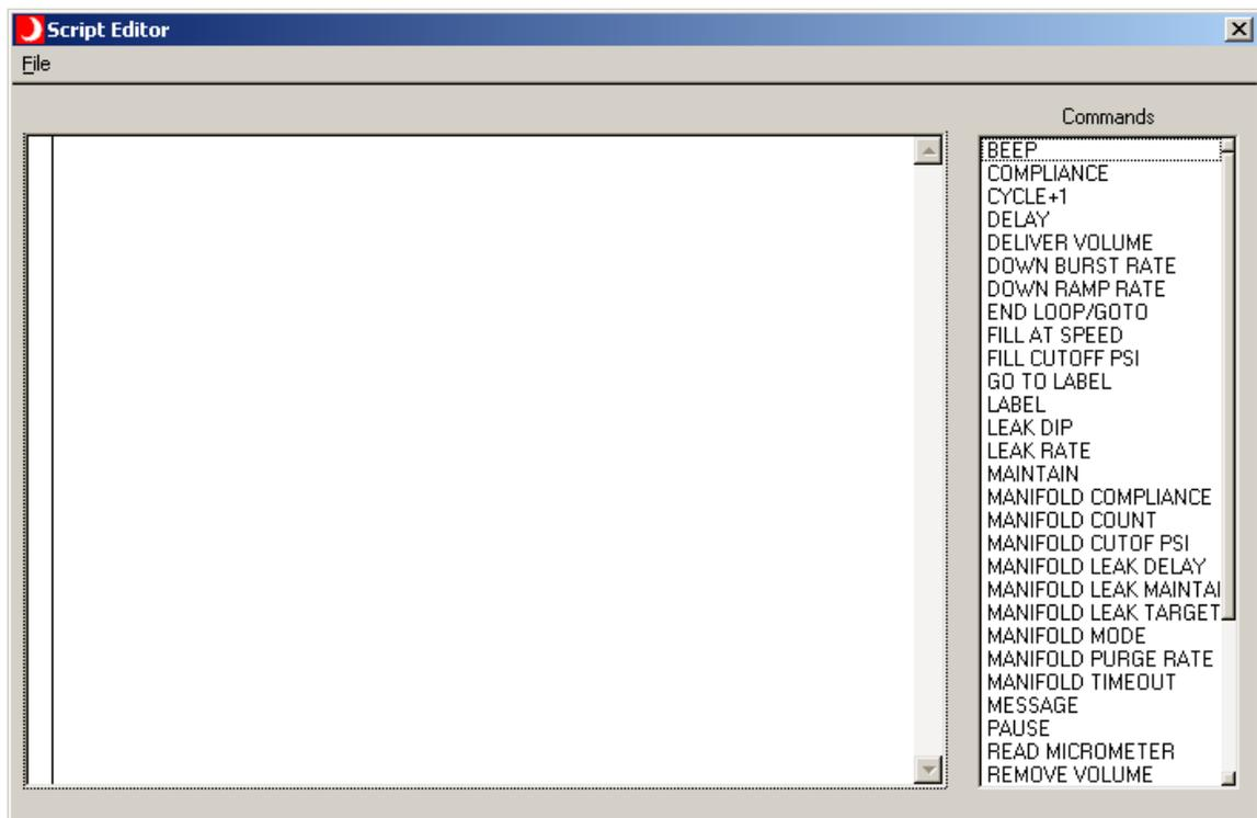
Use this panel to enter a new script or edit an existing script. The editor is content directed. That is the editor knows the syntax of the available script commands. The editor validates and completes the command syntax while the operator keys in new lines. The editor also checks parameter values based on HBLT pressure type and model type. In short, the editor insures that the operator enters only correctly formatted scripts.
