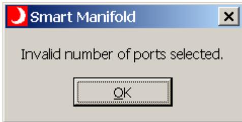
Cause: The user started a test with an invalid port combination selected on the Smart Manifold. Not selecting any ports or selecting more than one port when using single port mode causes this problem.
