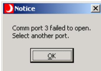
Cause: The HBLT port failed to open.
