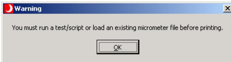
Cause: User attempted to print micrometer data before running a test or script.
