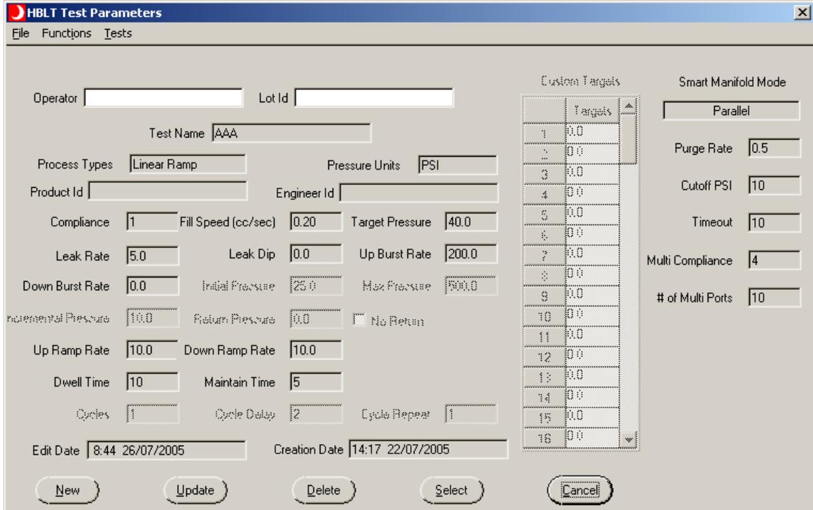
This version of the Test Parameters panel displays the Smart Manifold settings on the right hand side of the panel. These settings appear only when the HBLT has a Smart Manifold attached. If the Smart Manifold mode is parallel, the other Smart Manifold settings are active. Otherwise, the other controls are dimmed.
