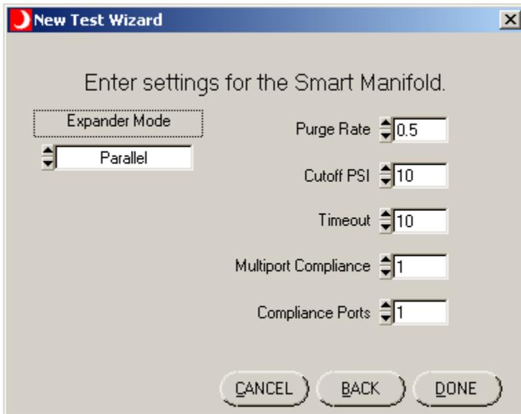
Use this panel to enter the parameters specific to the Smart Manifold.
