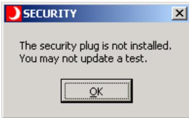
Cause: The Sentinel Pro security plug is not plugged into the parallel printer port or the USB port.
