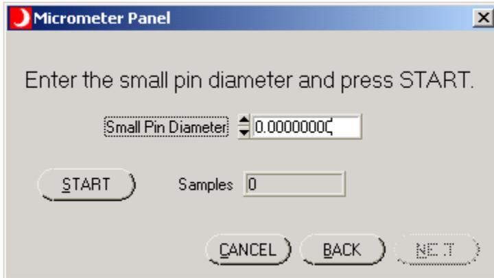
Use this panel to calibrate the small pin diameter.
