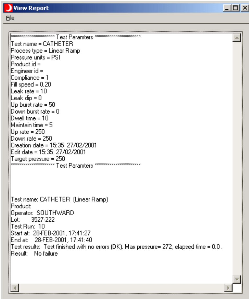
This panel displays the results of the current test. For HBLT tests, Pressure Manager displays the test parameters followed by the test results. For Pressure Manager scripts, Pressure Manager displays the script followed by the test results.
