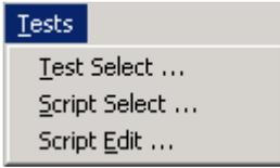
**Tests>>Test Select** This menu item opens the HBLT Test Parameters window to create, edit or select a predefined HBLT test.
