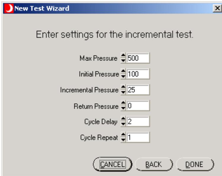
Use this panel to enter the parameters specific to the incremental test.
