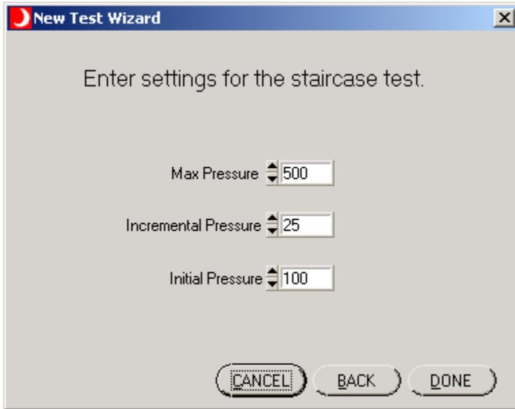
Use this panel to enter the parameters specific to the staircase test.
