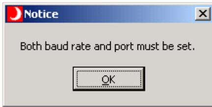
Cause: The baud rate or port is not defined correctly.
