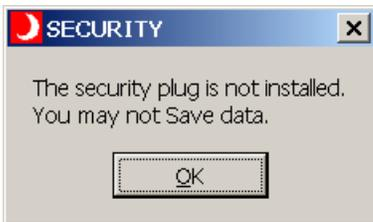
Cause: The Sentinel Pro security plug is not plugged into the parallel printer port of the USB port.
