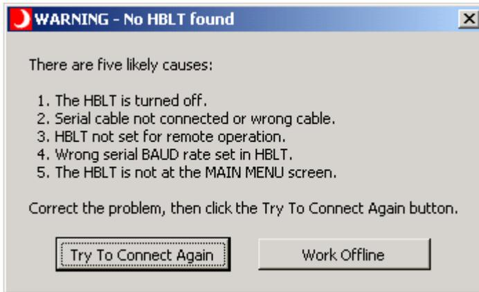
Cause: The basic cause is a failure to communicate with the HBLT. The five common errors that cause this problem are:
