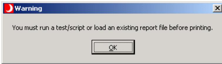
Cause: The report or log panel is empty. Run a test, script or open an existing report/log file before using the print command.
