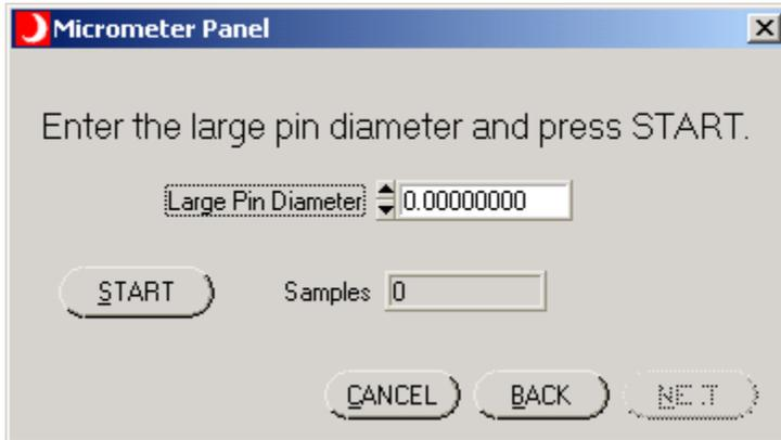
Use this panel to calibrate the large pin diameter.
