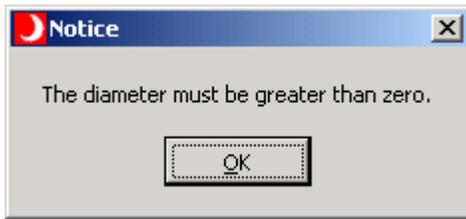
Cause: The small pin diameter is zero.
